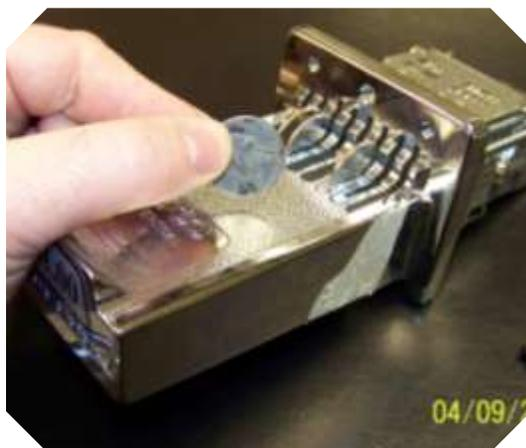
2) To gain access to the inserts, put your coins into the correct slots and then push in the handle.
