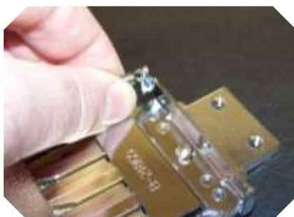
4) and unhook the two large return springs from the small hooks on the spring bracket.
