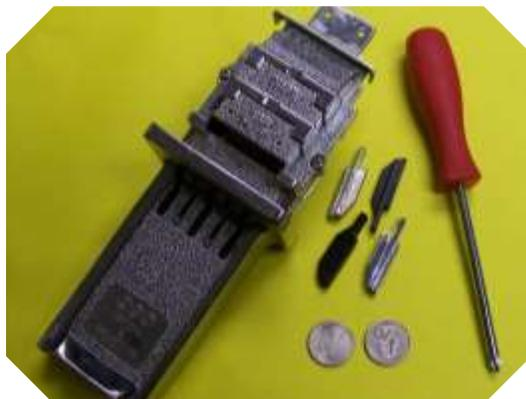
1) Remove the Push Chute from the coin door, and remove the push chute end, proximity plate, anything bolted to the end— for easier access. You will need the Push Chute (of course), enough coins to make it work in its current setting, the inserts for the desired setting, and a Phillips screwdriver.
