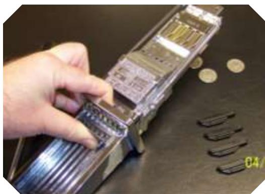
3) After pushing in the chute and your coins drop out, you will be able to access the inserts, and a section that may contain spare inserts. Continue to hold the handle in as shown...
