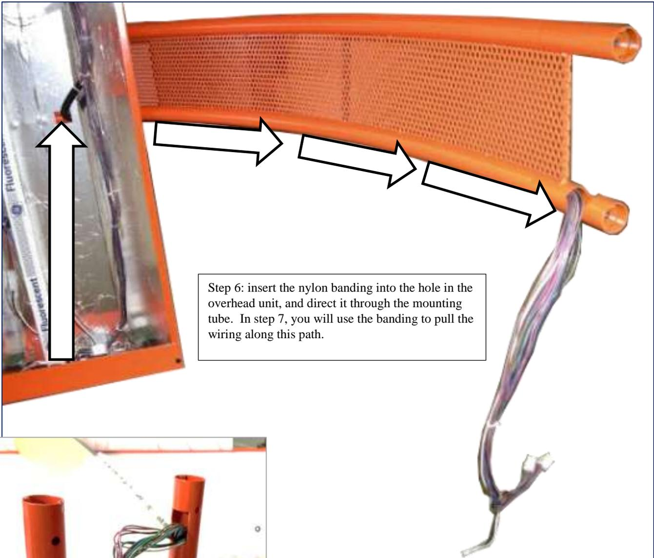
Step 6: insert the nylon banding into the hole in the overhead unit, and direct it through the mounting tube. In step 7, you will use the banding to pull the wiring along this path.
