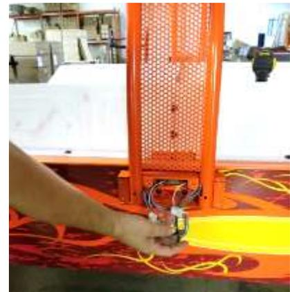
Step 12: On REAR side wall, feed the wire harness through the bracket opening.
