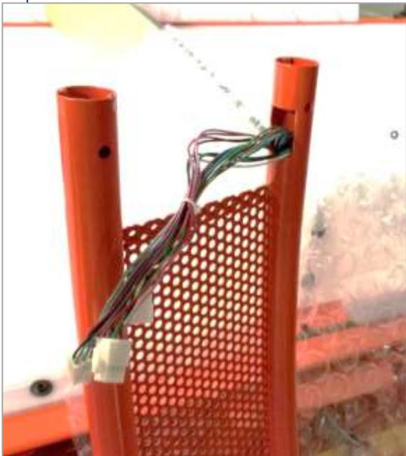
**6.** The Fire Storm overhead's unique design has narrower-diameter tubes than the standard overhead and it can be a challenge to feed the Overhead Wire Harness from the housing through the tube. We suggest taking a piece of the nylon banding used to box your overhead (or table). Insert the nylon banding into the SQUARE hole at the base and route it through the square hole in the top of the overhead housing.
