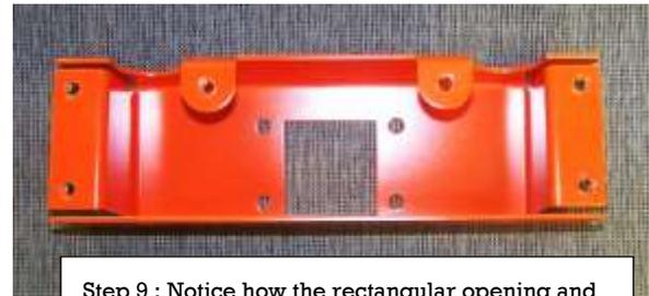
Step 9 : Notice how the rectangular opening and four bolt holes on the side of the table match the rectangular opening and four bolt holes found in the Side Mounting Bracket. Always install this bracket large holes UP, small holes DOWN
