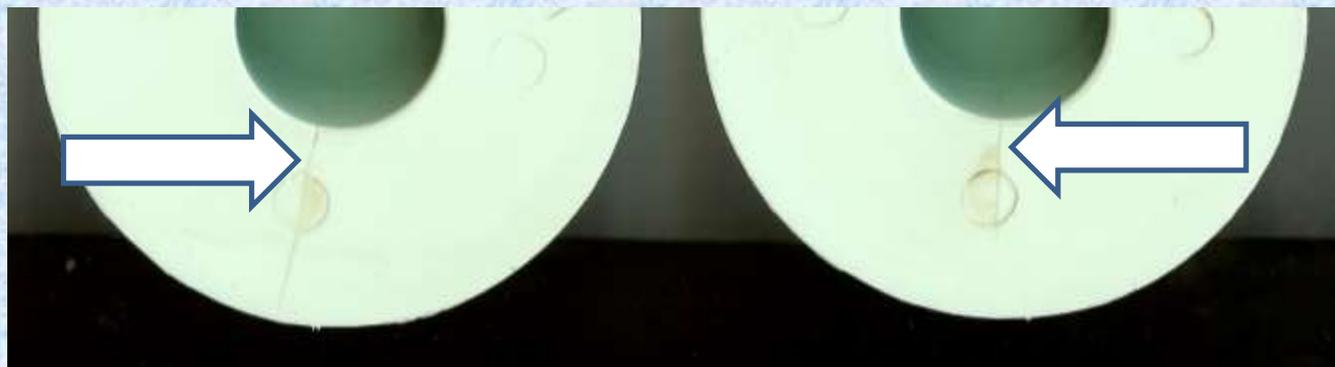
**ARE MY BRAND NEW MALLETS CRACKED? SEE THE FAINT LINE ON THE BOTTOM?** That's not a crack in the plastic, that's a surface line from the mold. It doesn't go through the plastic, doesn't affect the structural integrity of the mallet, won't affect performance, and will vanish instantly with a little rub of that [240 grit sandpaper](#).
