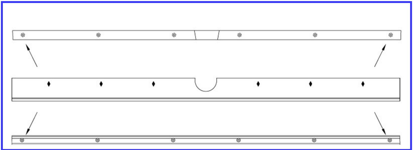
Drill the end mounting holes on the side rail using a  $\frac{3}{8}$ " diameter drill bit. From the cushion side, drill no deeper than  $1 \frac{3}{64}$ ". This will allow just enough movement of the rail bolt so it can be angled to attach to the current-model cushion rails.
