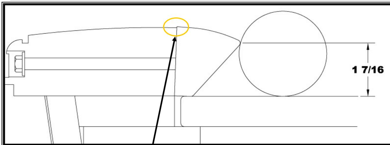
**THEY STILL LOOK A LITTLE HIGH TO ME:** Sometimes, the cushions may be as much as 1/16" higher than the rail laminate. **NOT A PROBLEM.** Rail height is measured from the slate surface up. If you set the cushions so they are flush with the rail laminate and ignore the crucial measurement from the slate surface, you increase the chance of balls bouncing over the cushions— and onto your players!
