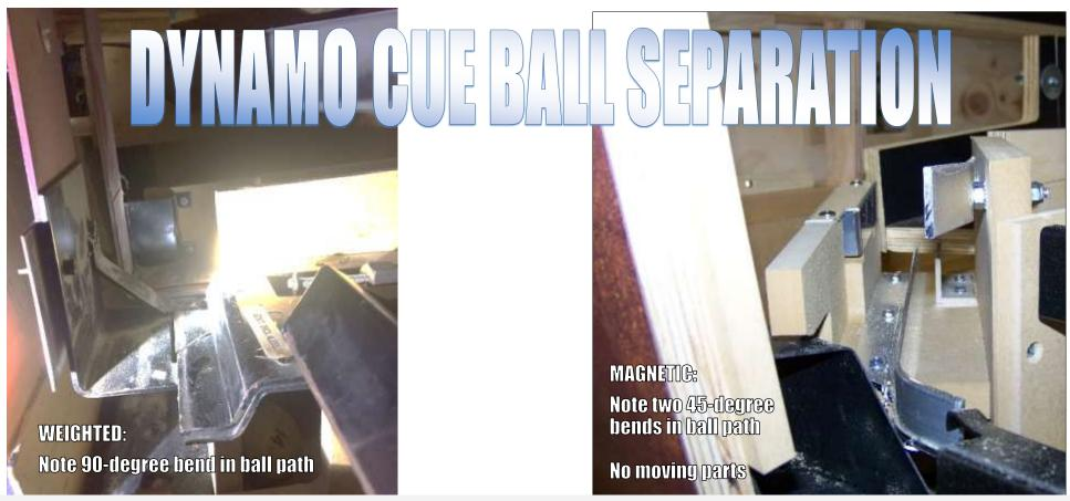
Prior to 1993—all Dynamo tables used WEIGHTED cue ball separation with a separator that looks like the photo on the left. We stopped stocking weighted cue balls over 10 years ago, but full-line parts suppliers have them. From 1995 to present—all Dynamo tables use MAGNETIC cue ball separation that looks like the photo on the right. From 1993—1995, it depends on what the dealer ordering the table specified.
