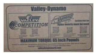
WHAT IS THE TORQUE SPEC FOR RAILS? We tighten rails to 65 inch-pounds (as we print on the box – here it is again), but for consistent quality play it is far more important that rails are properly aligned, also noted in the Valley Cushion Rail Service Bulletin. Rails do not need to be super tight, just snug (and tightening them super-tight risks breaking loose the threaded inserts, which is not a covered Warranty Issue because—AS SHOWN -- we even print on the boxes "Do not"
