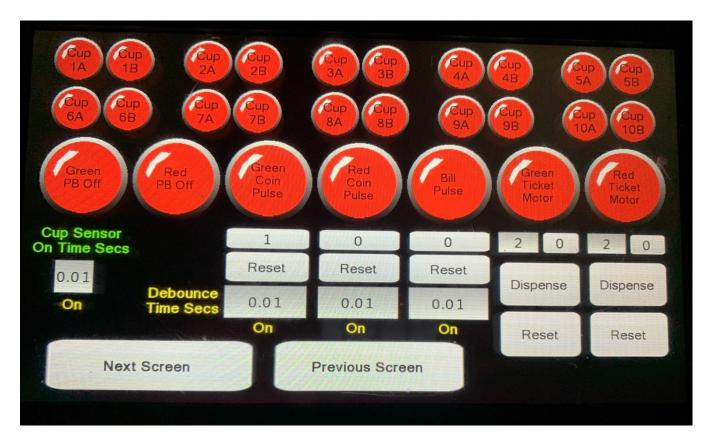
The pulse **"On"** time can be entered for the Green Coin, Red Coin and Bill Pulse. The fastest pulse time that you can enter is 0.01 seconds. The pulse **"Off"** time does not need to be entered.
