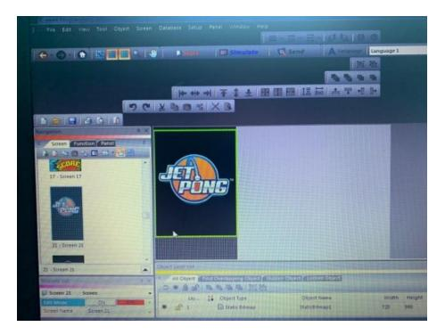
Press the Delete key on your keyboard. This will delete the Jet-Pong logo on Screen 21. Now along the top, press **"Object"**, **"Bitmap"**, **"Static Bitmap"**. Your pointer is now a +. Select the top left corner of the page that the logo was on and swipe down to the lower right. The Static Bitmap General tab should appear:
