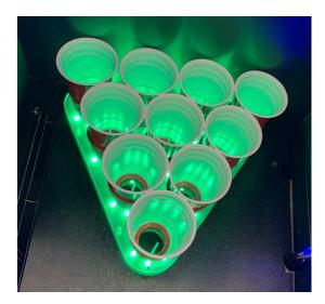
6) The Green LEDs under this cup should go out, cheering should occur and the rear Video Display should show a message for example GOAL!!! The rear Video Display and the HMI Touch Screen will then display which cup was made.
