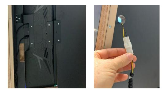
7) Connect the LED Strips to any Led Strip Cables connected to the SP901E Video Controller. Make sure they run through the black raceway and then close the tray covers.
