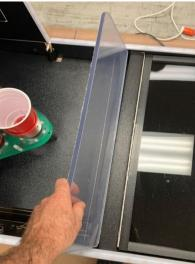
17) Remove the Protective Coating from the Side Shields. Using a 4mm or 5/32" hex Allen-key install the Side Shields using the screws provided in the Cash Box. Do not overtighten.
